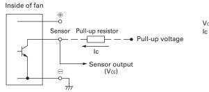
Vce = +27.6 V max. Ic = 5 mA max. [Vol = Vce (SAT) = 1.0 V max.]
