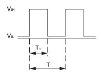
$V_{IH}=4.75$  to 5.25 V  $V_{IL}=0$  to 0.4 V PWM duty cycle (%) =  $\frac{T_1}{T} \times 100$  PWM frequency 25 (kHz) =  $\frac{1}{T}$  Current source (Isource) = 1 mA max. (when control voltage is 0 V) Current sink (Isink) = 1 mA max. (when control voltage is 5.25 V)
