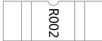
By mechanical trimming ( Front view )
