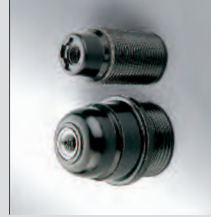
Thermostat lampholders: left, with E27 coupling, partly threaded skirt and metal nipple; right, with E14 coupling, fully threaded skirt and moulded thread.
