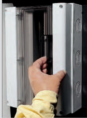
The semi-transparent tinted window, lockable and sealable. To open it, just lower the handle provided, snap-closing.
