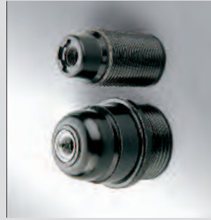
Thermoset lampholders: left, with E27 coupling, partly threaded skirt and metal nipple; right, with E14 coupling, fully threaded skirt and moulded thread.
