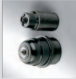
Thermosat lampholders: left, with E27 coupling, partly threaded skirt and metal nipple; right, with E14 coupling, fully threaded skirt and moulded thread.
