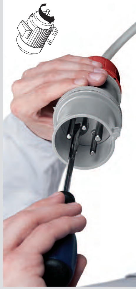
The phases are inverted by simply pushing and turning the phase pin support with a screwdriver.
