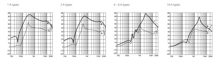
**FN 9290 B Series | Typical filter attenuation |** Per CISPR 17; A=50  $\Omega$ /50  $\Omega$  sym; B=50  $\Omega$ /50  $\Omega$  asym
