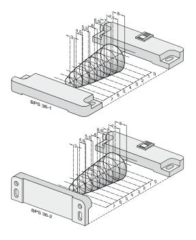
Assured switching distance:  $s_{ao} = 7 \text{ mm}$
