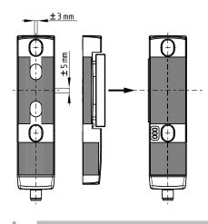
The safety component must be operated in the operating direction of the latching force (refer to image).
