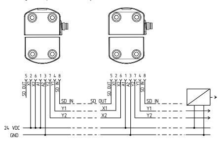
Y1 and Y2 = Safety outputs  $\to$  dual-channel safety monitoring module SD-IN  $\to$  Gateway  $\to$  Field bus
