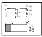
Representation of the contacts in non-actuated state (guard closed), switching angle in new state. Tolerance  $4^{\circ-2}$ .
