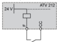
“PLC” position with PLC transistor outputs
