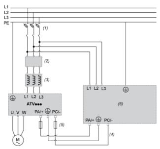
AC protection fuses Optional additional EMC input Filter (see drive catalog) Optional AC Choke (see drive catalog)
