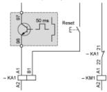
Associated components KA1: CAD + LAD6K10 or RHKKM1: LC1 D or LC1 F
