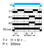
Function Qt: Star-Delta Relay (2 CO Outputs with Split Common)
