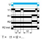
Function Ac: On-Delay and Off-Delay Relay with Control Signal
