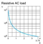
Switching capacity (kVA)
