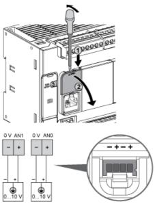
The (-) poles are connected internally.
