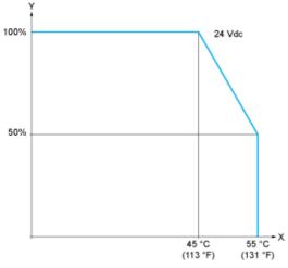
X: Ambient temperatureY: Input simultaneous ON ratio
