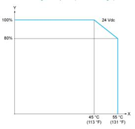
X: Ambient temperatureY: Input simultaneous ON ratio
