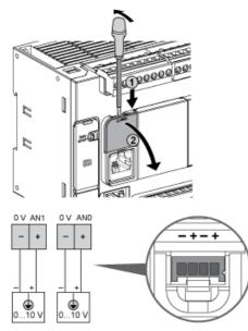
The (-) poles are connected internally.
