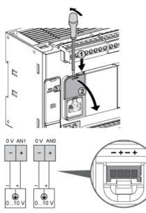
The (-) poles are connected internally.
