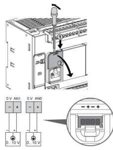
The (-) poles are connected internally.
