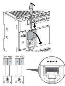
The (-) poles are connected internally.
