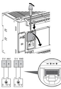
The (-) poles are connected internally.
