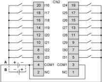
The COM0 and COM1 terminals are not connected internally
