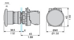
e: clamping thickness: 1 to 6 mm / 0.04 to 0.24 in.
