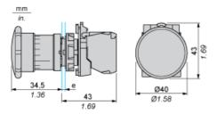
e: clamping thickness: 1 to 6 mm / 0.04 to 0.24 in.
