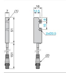
Coded magnet for XCSDMC XCSZC1
