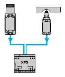
Locking of actuator and operation in positive mode associated with a safety module.
