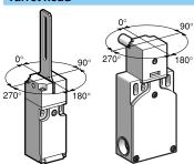
Safety switches for hinged covers or guards, featuring a hinged lever or spindle operator, incorporate a turret head that can be rotated through 360° in 90° steps. Two additional self-locking screws are included with each switch for positive fixing of the head.
