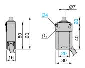
(1) Protective plate fixed by 5-lobe torque safety screws.
