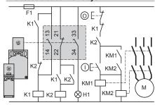
To activate K1, the lever or spindle must be rotated when the supply is switched on.
