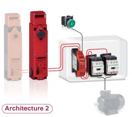
1 XCSLF (or series mounting) + XPSAC + 2 LC1D + 1 XB4 start + XPSVNE (for zero speed detection)
