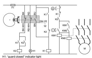
Example of guard monitoring using 2 switches and 1 safety module (PL=e, category 4 conforming to EN/ISO 13849-1) Operation in positive and negative (combined) mode
