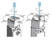
4 in the horizontal plane (1 for **XCSMP**), 4 from above the switch (1 for **XCSMP**), (4 alternative positions of the actuator slot, depending on the orientation of the head).
