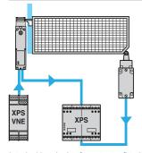
Interlocking device for actuator fitted on guard and zero speed detection.
