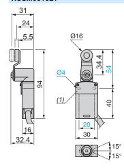
(1) Protective plate fixed by 5-lobe torque safety screws.
