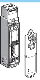
With the machine guard closed and locked, the resistance to forcible withdrawal of the actuator fitted to the guard is Fzh 2300 N according to the verification principle GS-ET19 (Fzh=Fmax/1.3). In addition to the 3-pole contacts, positively operated by the actuator fitted to the guard, safety interlock switches XCSLF incorporate NC + NO or 2 NC or 1 NC + 2 NO or 2 NC + 1NO or 3NC contact blocks mechanically linked to the solenoid.
