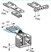
Their oblong fixing holes enable simple adjustment when mounting on moving guards.
