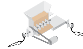
Detection of underspeed, shaft overload
