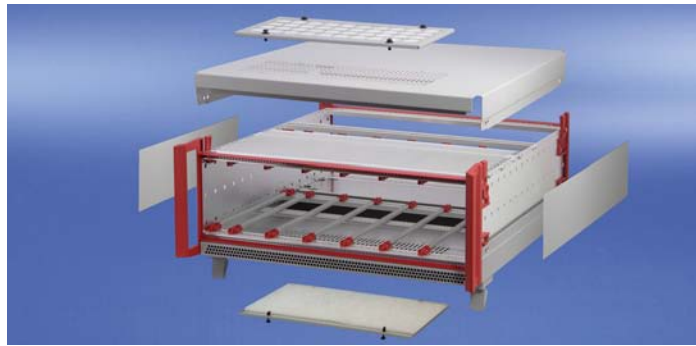
Application: ratiopacPRO-air case in special colour, shielded board cage, filter mat top and bottom
