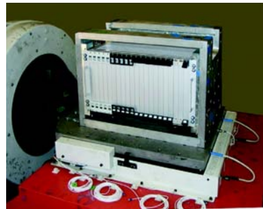
Y-axis_001a1 Shock and vibration resistant in all three axial directions
