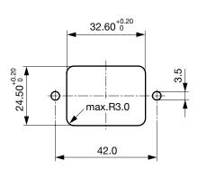
A = 32.0 mm; quick-connect terminals 6.3 x 0.8 mm A = 30.4 mm; quick-connect terminals 4.8 x 0.8 mm
