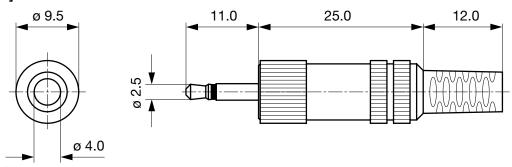
Cable diameter max. 4.0 mm
