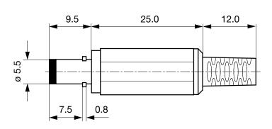
Cable diameter max. 4.0 mm
