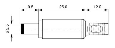
Cable diameter max. 4.0 mm
