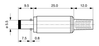
Cable diameter max. 4.0 mm
