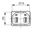
E: Solder terminals 22.5 mm E:Quick connect terminals 25.5 mm S: 1.0, 1.2, 1.5, 2.0, 2.5, 3.0 mm
