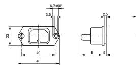
E: Solder terminals 20.5 mm E: Quick connect terminals 23.5 mm
