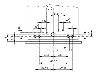
Fixation on PCB or housing from below
