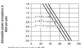
Ambient air temperature Ta  $^{\circ}\text{C}$
