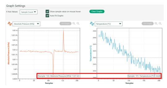
Auto Fit Graphs: when deactivated, the functions Fit Graph, Zoom In, and Zoom Out will become enabled. Move the cursor to the graphs and, while holding Alt, click and drag the mouse to create a zoom region to zoom into and check sensor performance in detail. To zoom out click the Fit Graph icon.
