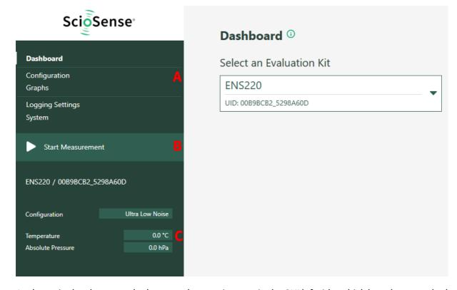
As shown in the above graph, there are three main areas in the GUI left side, which have been marked accordingly with three red letters A, B, and C. These three areas Am, B, and C have been defined as below:
