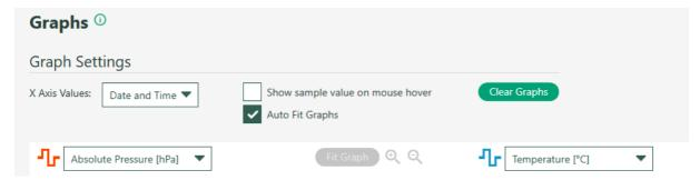
**Graph Settings:** With one drop-down menu and two checkboxes to choose the user's preferred way of data visualization, together with a button to clear the graphs.
