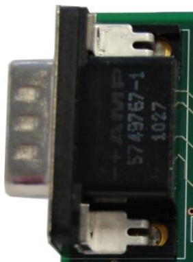
Figure 2.3: 15-pin VGA connector for power supply
