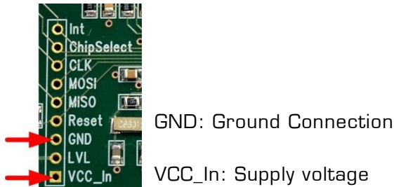
Figure 2.5 External power supply via J19
