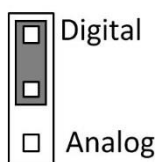
Figure 2.13: Jumper settings for analog/digital enable
