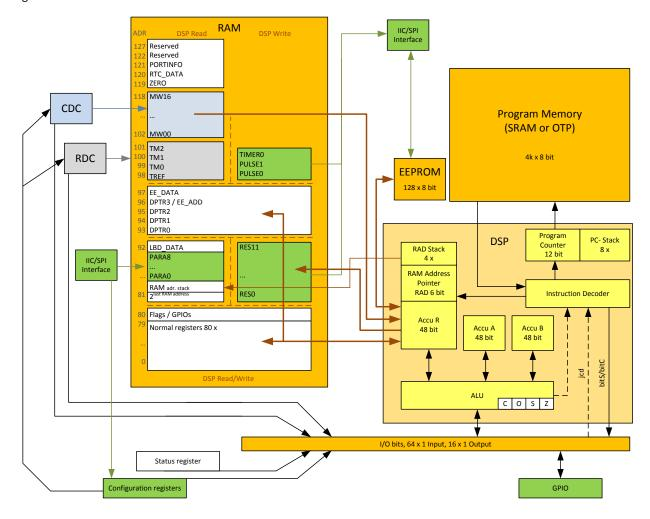
This Harvard DSP for 48 bit wide parallel data processing is coupled to a 128 x 48 bit RAM, 80 x 48 bit thereof free accessible. In read access, the DSP can get the CDC measurement raw data from address space 102 to 118, the RDC raw data from address space 98 to 101. By write access the DSP provides the output data to either the serial interfaces (addresses 81 to 92) or to the PDM/PWM interfaces (addresses 98, 99).
