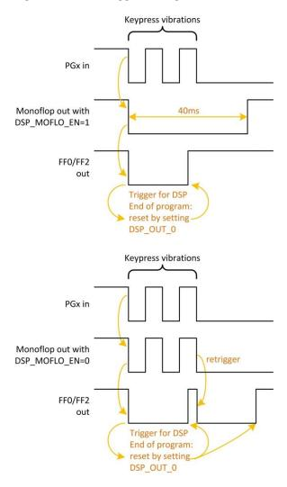
There is a possibility to activate a 40 ms debounce filter ("monoflop") for the ports in case these are used as inputs. This might be useful especially in case the DSP is started by the pins (signals FFO, FF2). Figure 2-3 shows the effect of the monoflop filter.
