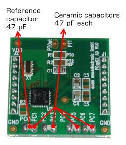
Figure 2-2: Details of the plug-in module
