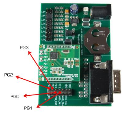
Figure 2-4: General purpose interface ports PGO to PG3
