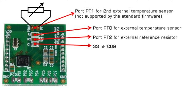
Figure 2-3: Temperature sensor connection pads
