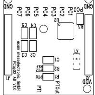
Figure 4-3: PCaO2 AD module layout
