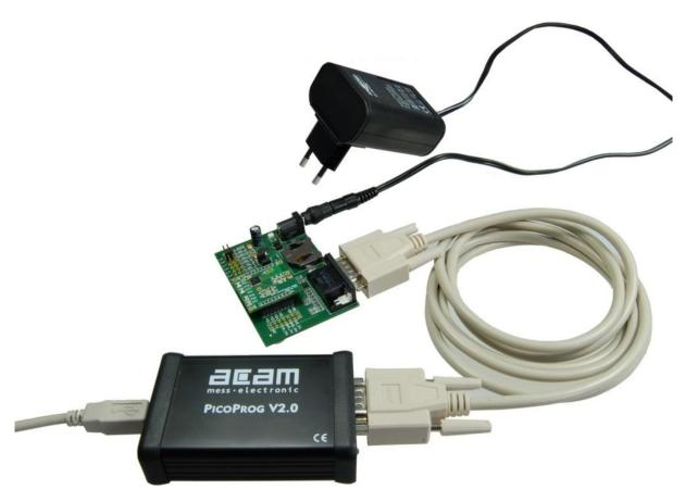
Figure 1-1: Components of the evaluation kit
