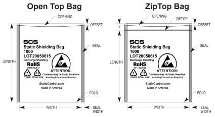
Tolerance: Width -0, +1/4" Length +/- 1/8" Offset 0 to 1/4" Seal width 3/8" with a tolerance of +/- 1/8" Note: Standard bag markings shown above and are not to scale.
