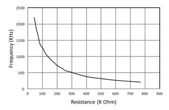
Figure 5. Switching Frequency vs FSW Resistance
