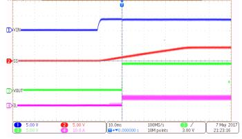
Figure 18. Switching Waveforms in PFM
