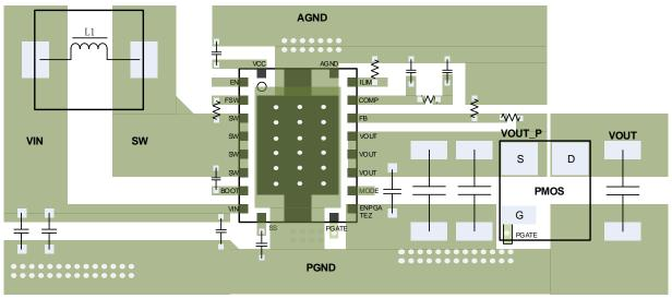
Figure 26. PCB Layout Example Top Layer
