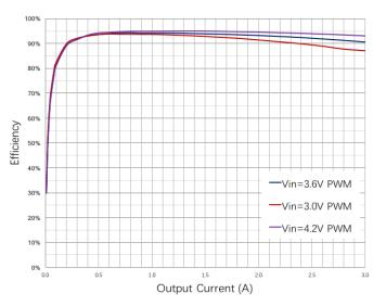
Figure 2. Efficiency, Vout=9V, fsw=560KHz, PWM
