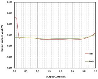
Figure 11. Load Regulation (Vin=3.6V, Vout=9V)
