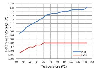
Figure 10. Feedback Reference Voltage vs Temperature
