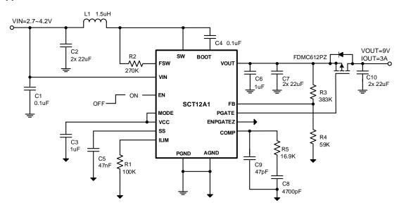
Figure 15. One Cell Battery Input, 9V/3A (30W) Output with Load Disconnection Protection
