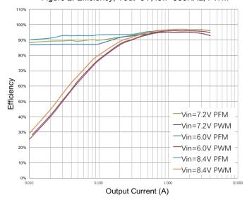
Figure 4. Efficiency, Vout=12V, fsw=560KHz, 2-cells Battery
