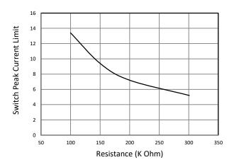
Figure 6. Inductor Peak Current Limit vs RLIM Resistance
