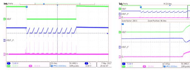
Figure 22. PSM, Output Hard Short with 0A Load
