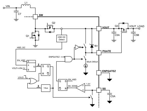
**Figure 13. Load Disconnection Control**
