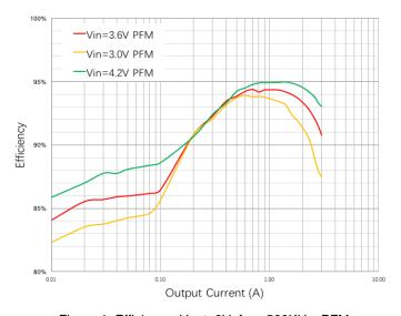
Figure 1. Efficiency, Vout=9V, fsw=560KHz, PFM
