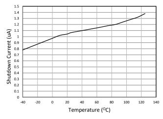
Figure 9. Shutdown Current vs Temperature
