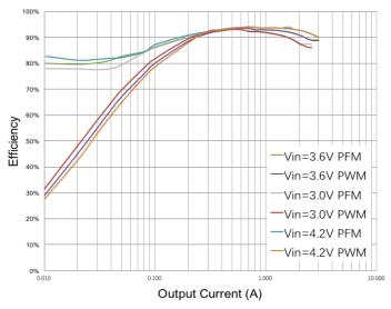
Figure 3. Efficiency, Vout=12V, fsw=560KHz, 1-cell Battery
