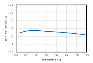
Figure 11. EN Threshold vs Temperature
