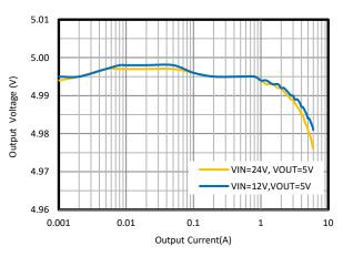
Figure 6. Load Regulation (Vout=5V)
