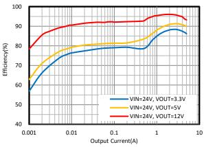
Figure 4. Efficiency vs Load Current, Vin=24V
