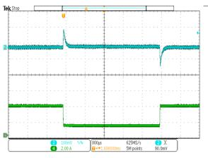
Figure 24. Load Transient (1.25A-3.75A, 250mA/us)
