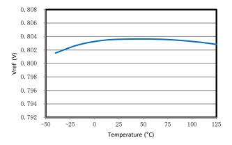
Figure 13. Reference Voltage vs Temperature
