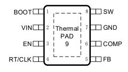
Figure 2. 8-Lead Plastic E-SOP
