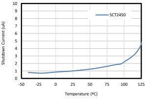
Figure 9. Shutdown Current vs Temperature
