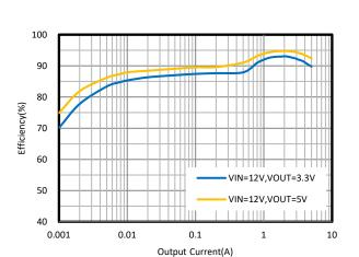
Figure 5. Efficiency vs Load Current, Vin=12V
