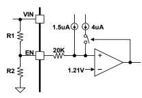
Figure 16. System UVLO by enable divide
