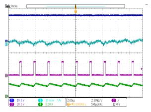
Figure 25. SW and Vout Ripple
