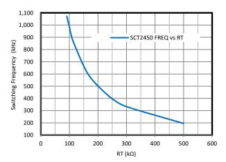
Figure 8.Clock Frequency vs RT/CLK Resistor
