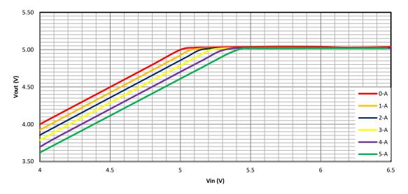
Figure 18. LDO Operation Characteristic (Vout =5V)
