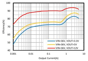
Figure 3. Efficiency vs Load Current, Vin=36V
