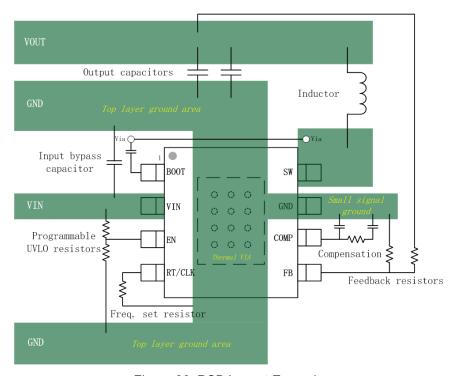
Figure 26. PCB Layout Example
