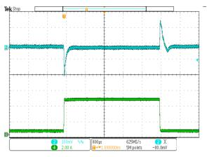
Figure 23.Load Transient (0.5A-4.5A, 250mA/us)
