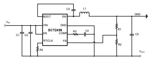
Figure 20. SCT2459 Inverting Power Supply
