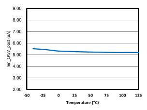
Figure 12. EN Pull-up Current vs Temperature
