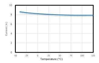
Figure 14. Peak Current Limit vs Temperature
