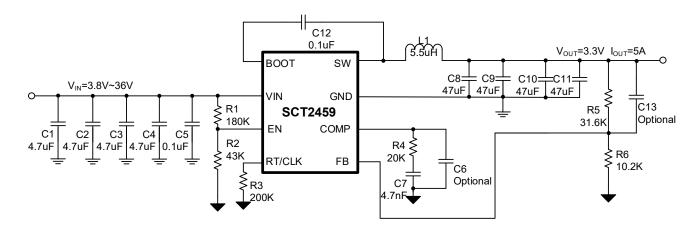
Figure 19. SCT2459 Design Example, 3.3V Output with Programmable UVLO
