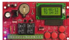
SA-027Q 365-Day Annual Timer • 2 Form C relay outputs • 100 Programmable events • Block programming • Built-in LCD display
