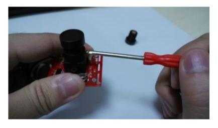
Try rotating the lens, it can be screwed out:
