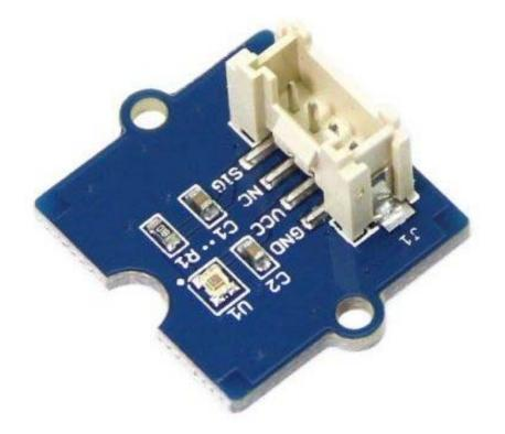
Grove - Luminance Sensor detects the intensity of the ambient light on a surface area. It uses **APDS-9002** analog output ambient light photo sensor. This has responsivity closer to human eye.
