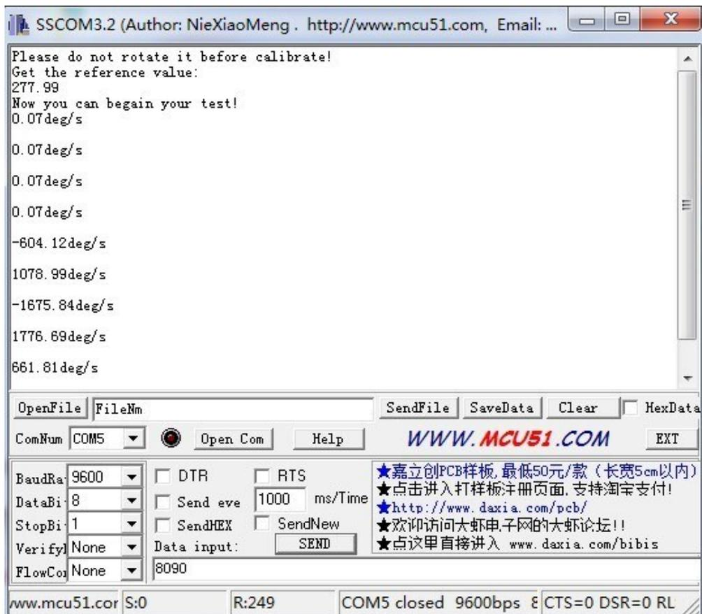
5. As you see the "Now you can begin your test", that means the calibration done. You can use the sensor now. Rotating direction can reference the following picture:
