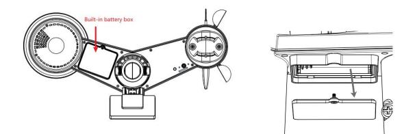
**Step 5:** Insert the dummy battery to the battery compartment, make sure the "OUTSIDE" marking faces outside and the +/- polarity in correct orientation.
