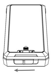
Step 4: Unscrew the battery door at bottom the of weather station.
