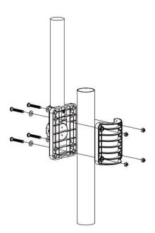
**Step 2:** Apply 2 rubber pads on the inner sides of the mounting base and clamp of the weather station, and loosely fasten them together.
