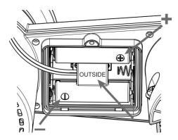
**Step 6:** Replace with the battery door which come along with the external battery box, then tighten the battery door screw. Once the installation completed, the red LED indicator at the bottom of the weather station will be flashing.
