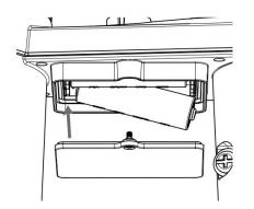
**Step 3:** Tighten the battery door screw. Once the installation completed, the red LED indicator at the bottom of the weather station will be flashing.
