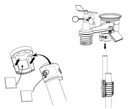
**Step 3:** Place the weather station over the mounting pole and align it to North direction before fastening the screws.
